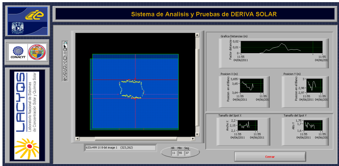
Figure 17. Front end of the solar spot test.
