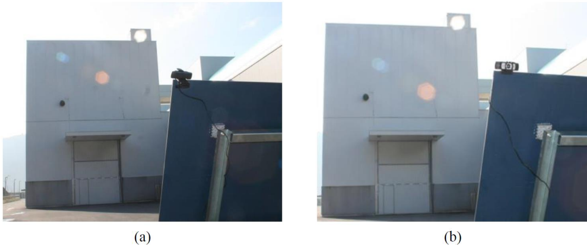
Figure 98. Camera mounted on a heliostat (a) Forward and (b) backward configuration.
