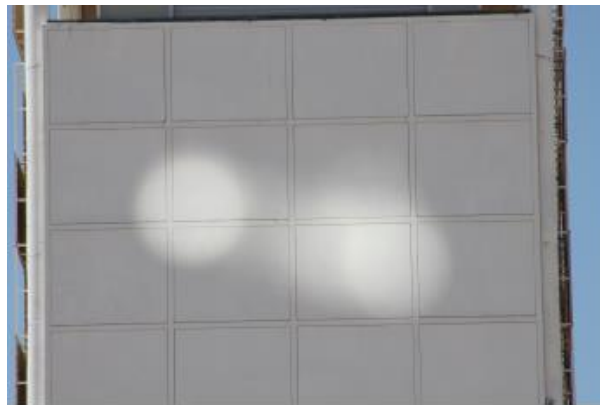
Figure 41. Image captured during the reflected spot test at 120 m distance.
