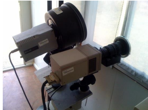
Figure 7. CCD camera ORCA II.
