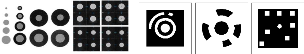
Figure 56. Retro-reflective targets (Coded targets preferred, circular targets, hard-body tooling targets).
