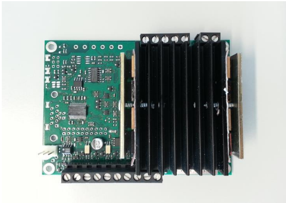
Figure 39. Electronic board of the stepper motor driver.
