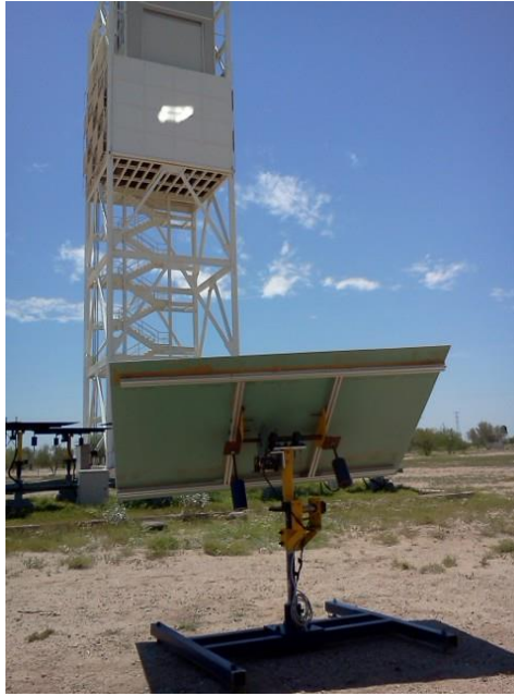
Figure 40. Heliostat of 1.5 m 2 reflecting the sun at 40 m distance.
