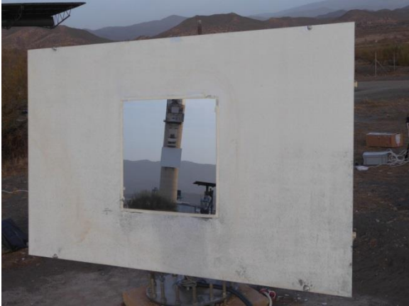
Figure 22. Reduced optical area of facet to focus on tracking accuracy.
