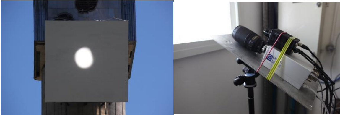
Figure 3. Camera set for the characterization of a heliostat at Themis.
