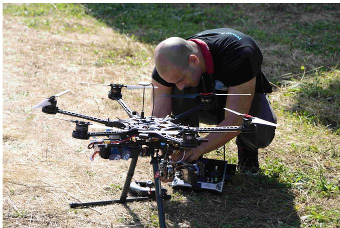
Fig. 21. Hexacopter by Nuova Sistemi Srl equipped with a Nikon AW1 compact camera.
