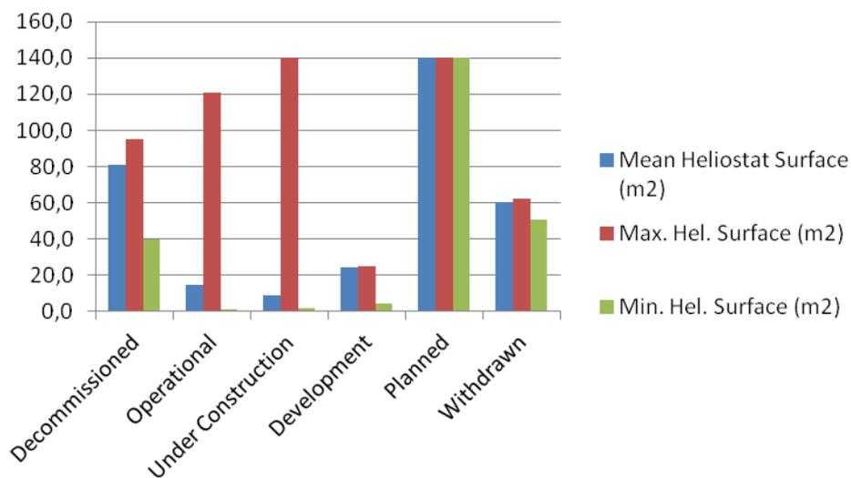
**Figure 18. Heliostats sizes by project status.**
