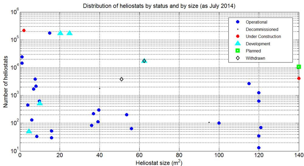
Figure 16. Distribution of number of heliostats deployed worldwide by project status and heliostat size.
